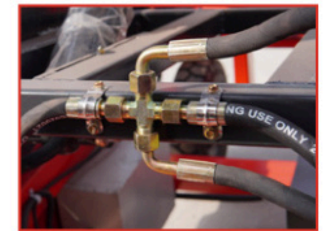
Oil pipeline layout
