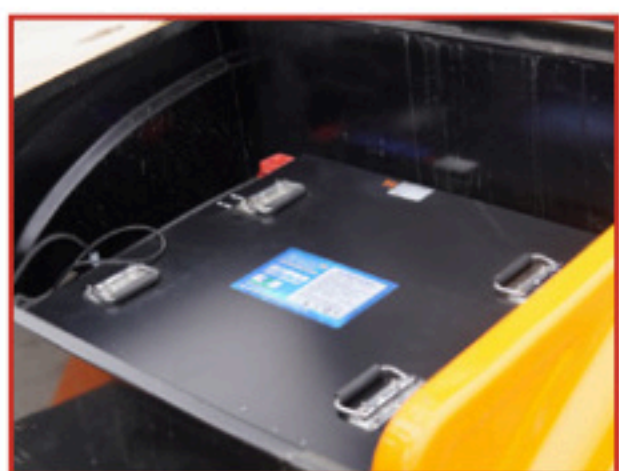
Large capacity battery pack
